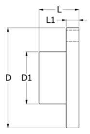
$\begin{array}{lll} D & = 105 \\ D1 & = 53 \\ L & = 45 \\ L1 & = 13 \\ Max \ bore & = 32 \\ Torque \ (N \ m) = 200 \end{array}$
